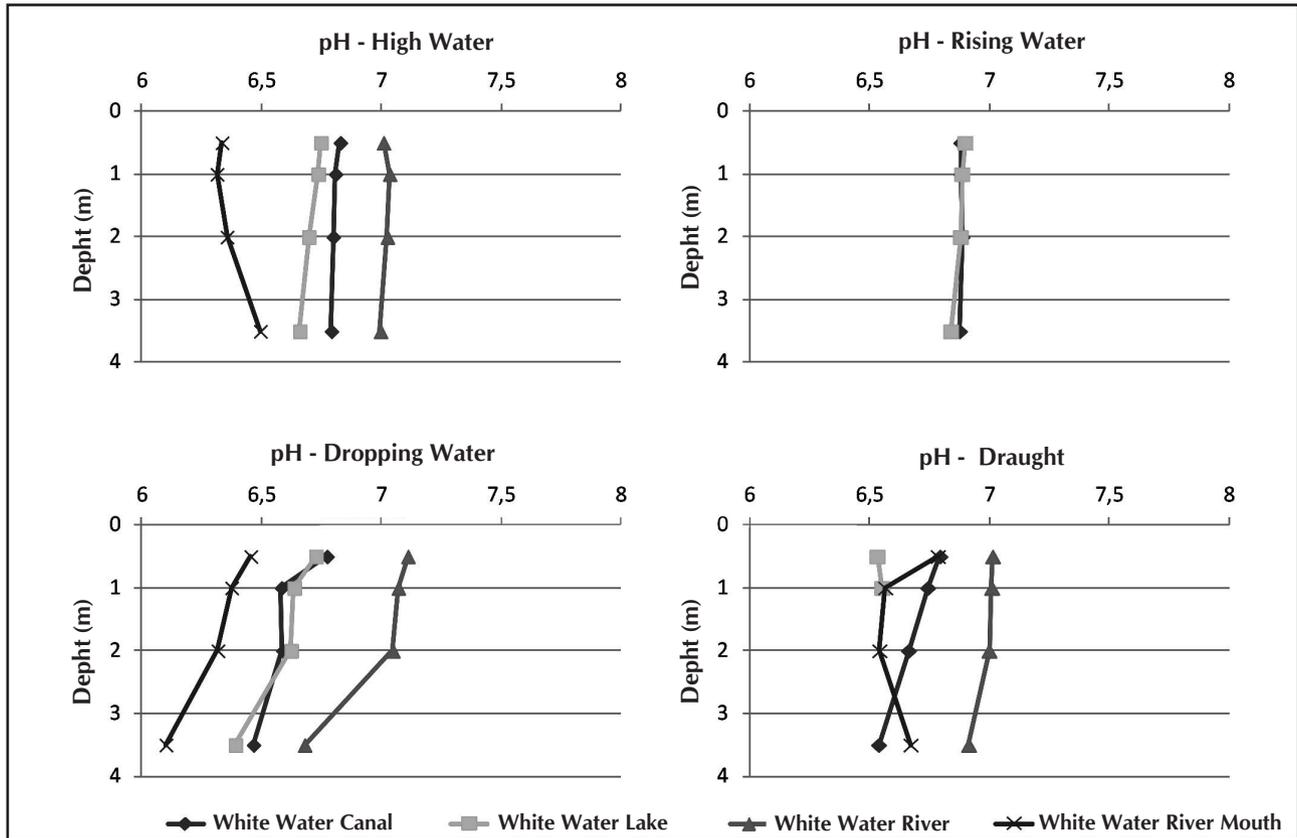
Figure 4 – pH measurements of water bodies during different periods of the hydrological cycle, by depth (m).
