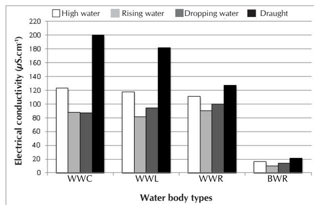
Figure 2 – Electrical conductivity ( $\mu\text{S}\cdot\text{cm}^{-1}$ ) of water bodies in different periods of the hydrological cycle.
