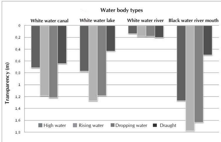
Figure 3 - Transparency (Secchi disk, in meters) of water bodies during different periods of the hydrological cycle.
